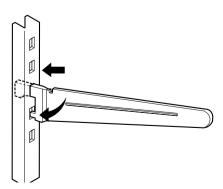
▲ CAUTION: Make sure that shelves are level from one side to the other. Failure to do so may result in the shelf falling or spilling food.
